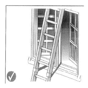
Ladder tied at the top stiles (correct for Tying part way down working on, but not for access)
